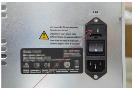
Fuse drawer with fuse 4 AT
