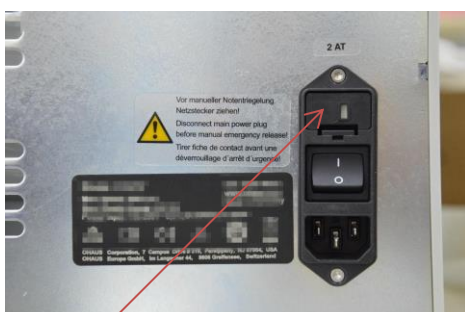
Fuse drawer with fuse 4 AT
